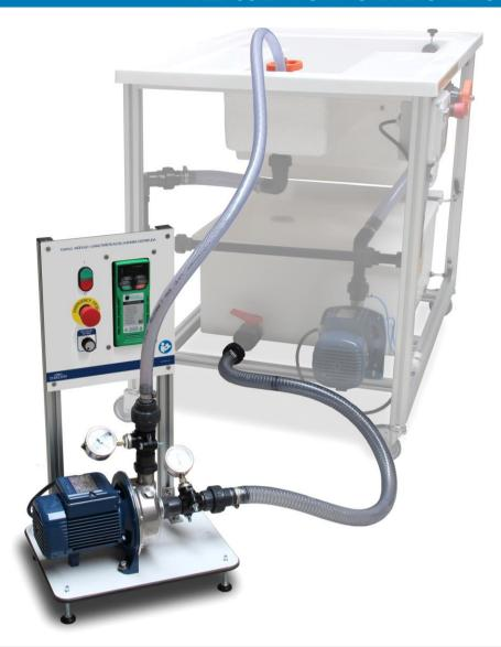
Pumps are included in a pipe system to convert mechanical energy into hydraulic energy. This additional energy allows the transmission of a fluid from one place to another when it is not feasible to flow by gravity, raise it to a certain height on the pump or recirculate it in a closed system. In general, the effect of a pump on a system is to increase the total energy by an H amount.
